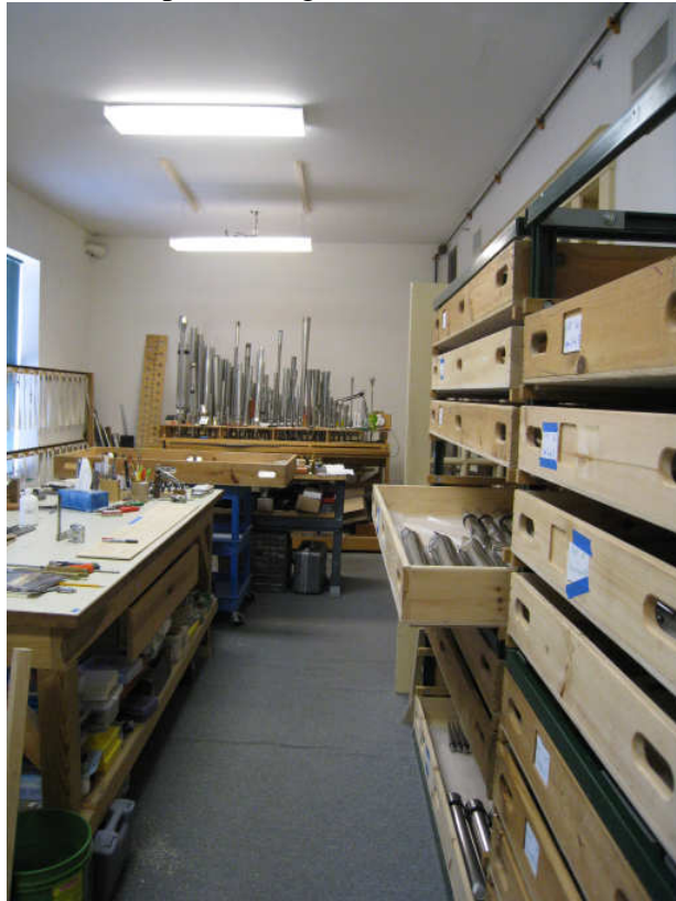
Pipes Staged in Voicing Room
