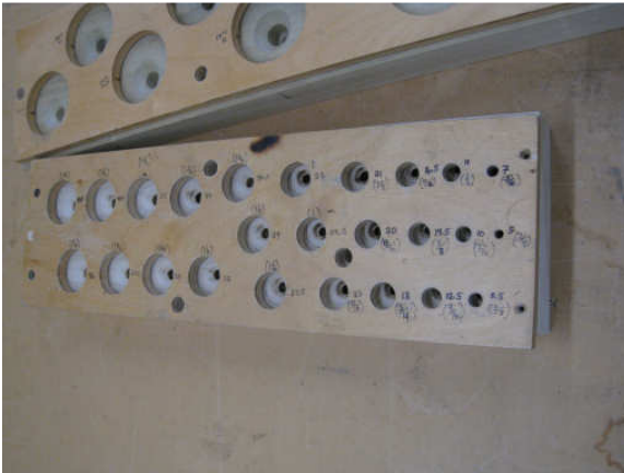
Templates for Making Pipe Racks
