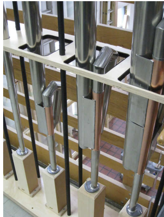
Racked Reed Pipes: 16' Boots and Mitered Resonators
