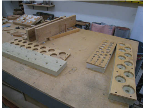
Templates for Making Pipe Racks
