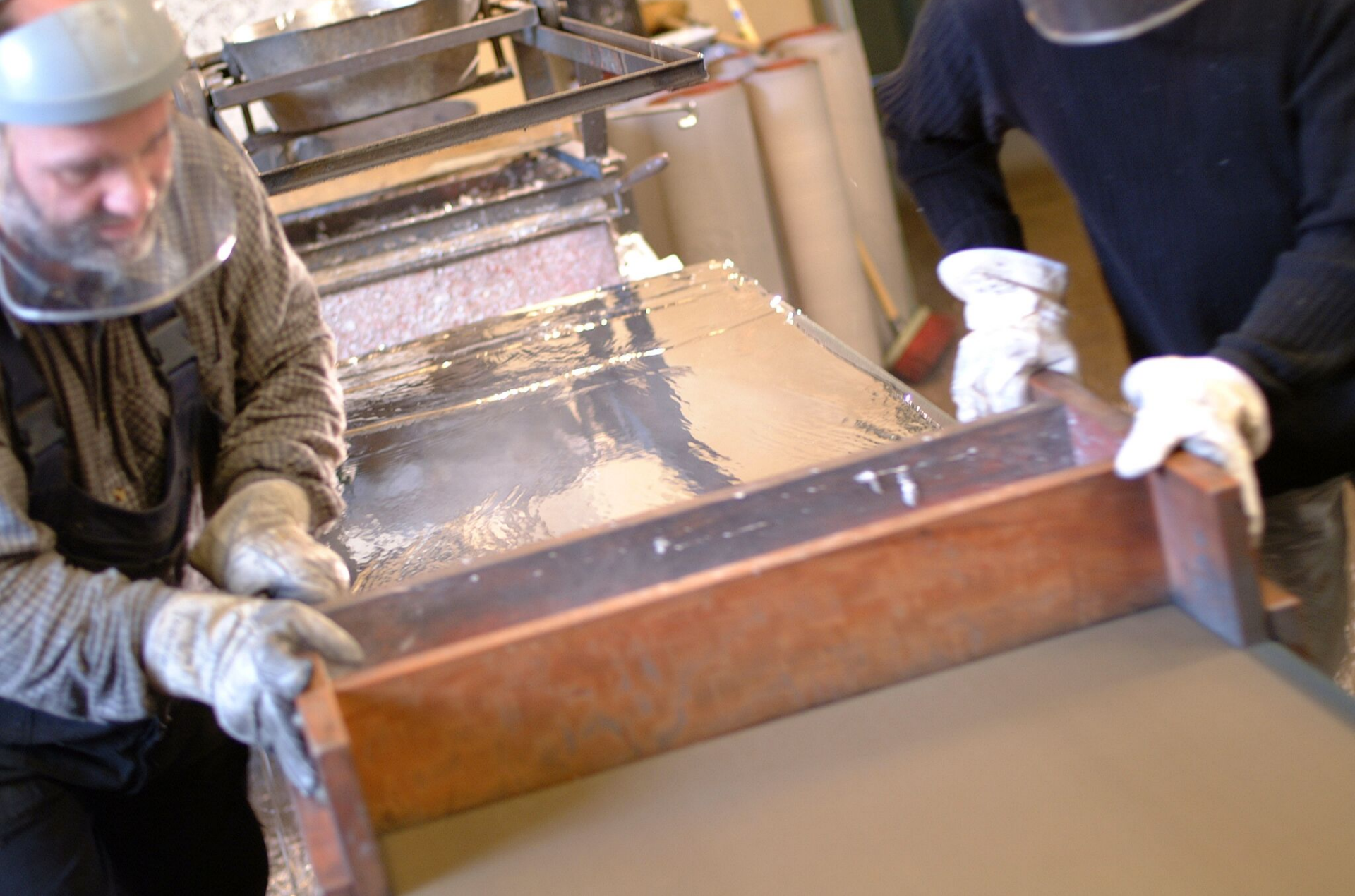
Two craftsmen slide the box along a counter as the metal runs out the slit creating a thin layer of metal.
