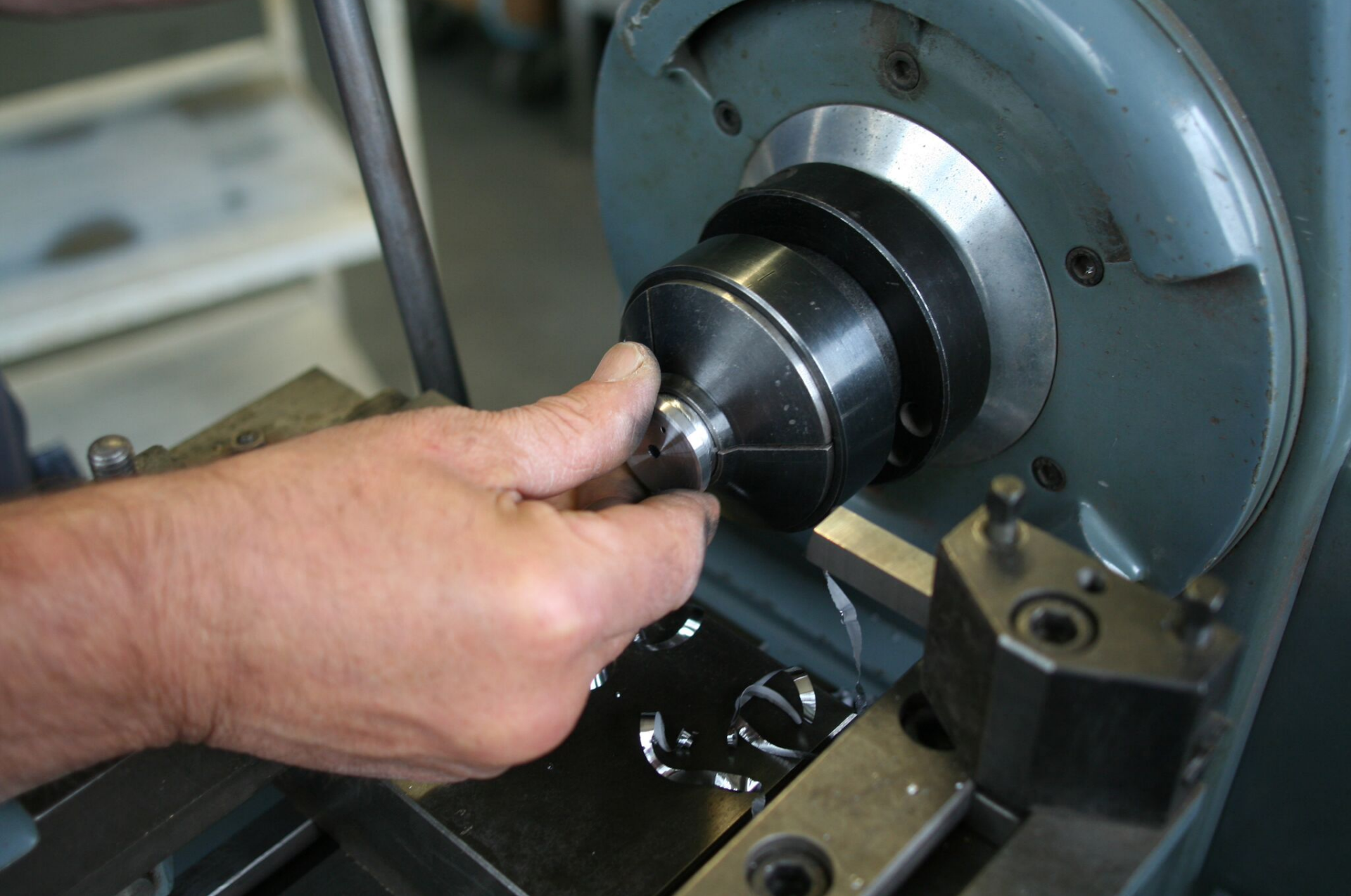
Here the resonator boxes for reed pipes are being machined.
