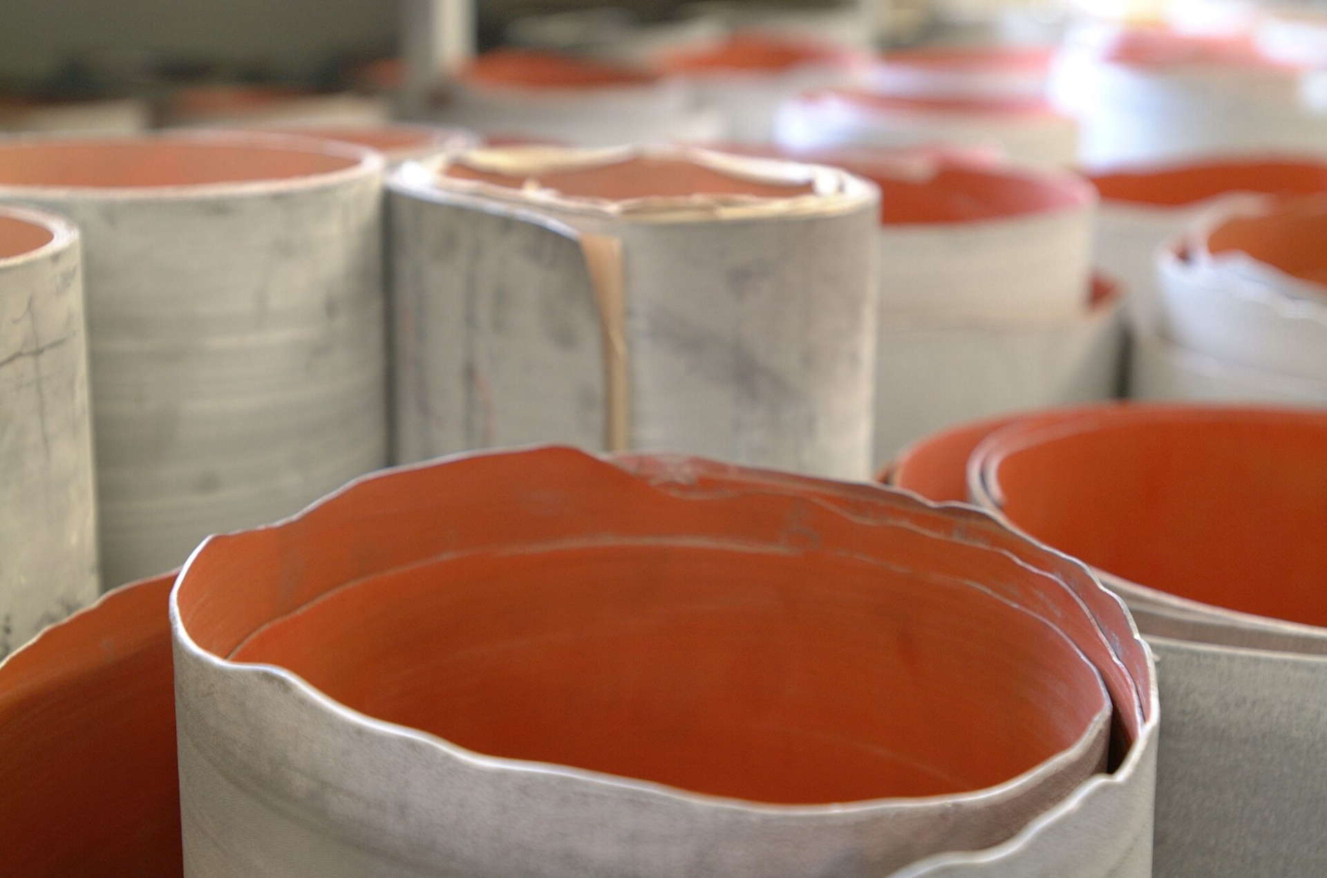
Metal organ pipes for Pilgrim's new organ being made by hand by Killinger Pfeiffen Freiberg, of Freiburg, Germany
